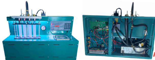
Figure 4: Real pictorial view for the gasoline injector cleaner device (left) rear view (right).
